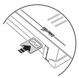
The LightCorder does not work with all flash memory cards. It will work with cards that you order from Martin, or cards from Toshiba and Samsung. Cards in the following sizes can be used 4 MB, 8 MB, 16 MB, 32 MB, and 64 Mb.
